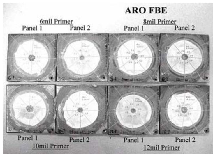
**Figure 6: To evaluate the effect of primary coating thickness of a DLFBE abrasion resistant outer-coat (ARO) system, a 65°C, 28 Day, -1.5 V, 3% NaCl cathodic-disbondment test was performed. With a total thickness of 525 µm, the primer thickness did not show an effect on cathodic-disbondment performance over the range of 150 to 300 µm. Photo courtesy of M. Dabiri**
