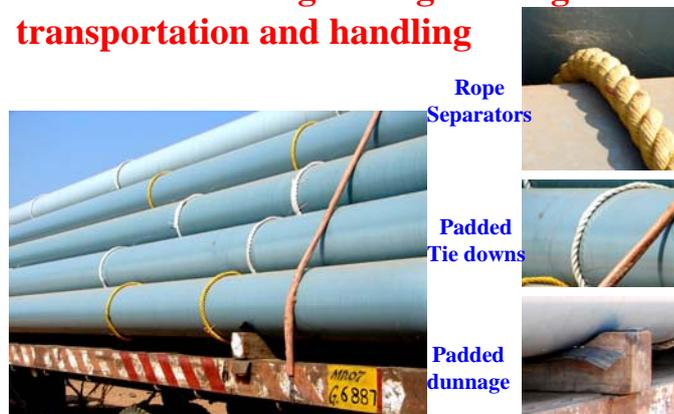
Figure 14: A well written specification requiring the use of separators, padded or non-damaging strapping, and correctly sized and padded dunnage will reduce the potential for coating damage. Photos courtesy of J. A. Kehr.
