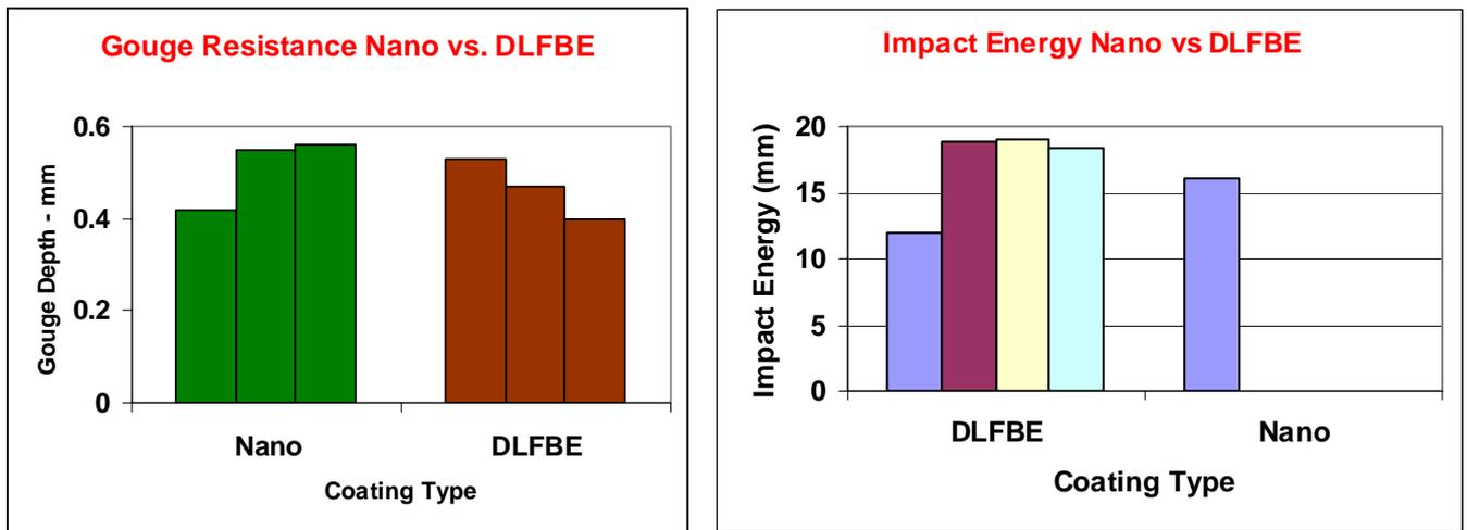
**Figure 17: Gouge and Impact Resistance of Nano DLFBE is similar to a standard DLFBE**
