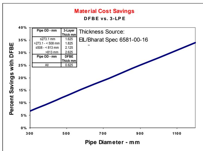
**Figure 11: Material costs of DLFBE and 3-layer coatings depend on pipe diameter. This is an example from India showing that the larger PE thickness required for larger diameter pipe significantly affects cost.**
