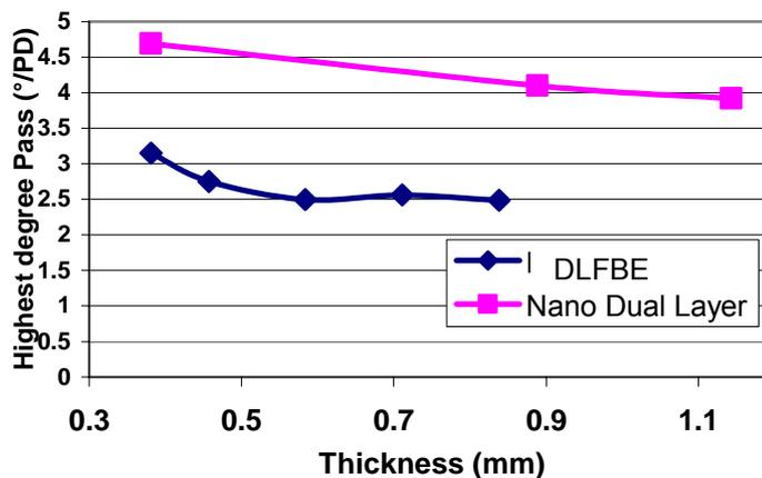
Figure 16: Nanotechnology has allowed a DLFBE to reach 4°/PD at -30C even at high thickness. This higher thickness can lead to more damage resistance without sacrificing flexibility
