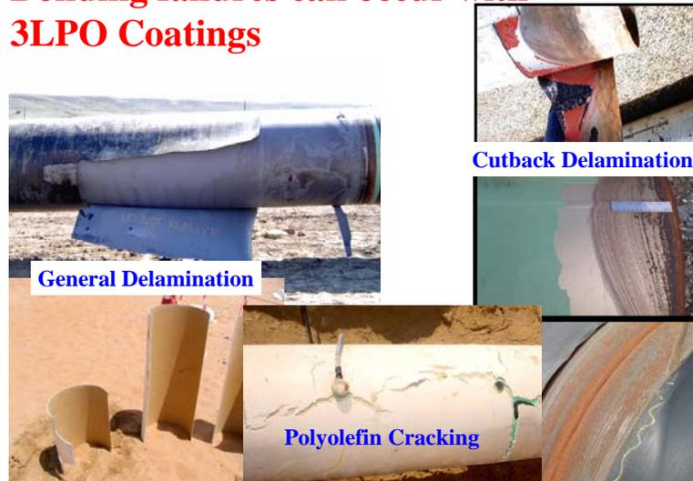
**Figure 8:** There have been numerous cases of disbondment with 3-layer polyolefin coating systems. That is significant because the high electrical resistance of polyolefins means that they shield the pipe surface from cathodic protection. There have also been cases of cracking after a few years of service.<sup>5,7</sup> Photos courtesy of D. Norman and A. Moosavi.
