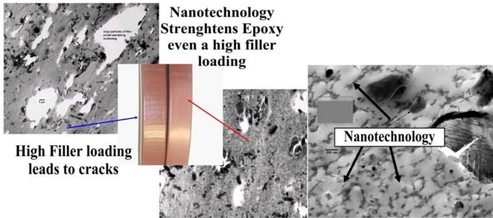
Figure 15: DLFBEs have been known to have reduced flexibility at colder temperatures. One practice in the industry to get better flexibility is to decrease filler loading. Decreasing filler loading decreases damage resistance (gouge and impact). Using nanotechnology has addressed the compromise between damage resistance and flexibility without decreasing filler loading. Nanotechnology strengthens epoxy even at high filler loading. Photos courtesy of M. Mallozzi
