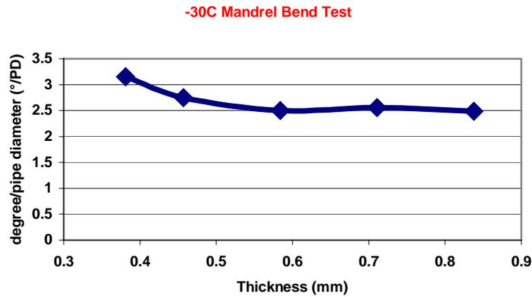
**Figure 5: As thickness of a DLFBE coating increases the flexibility slightly decreases reaching a minimum flexibility of about 2.5°/pipe diameter when coated at 0.8 mm. In each case, thickness of the primer corrosion coating was 0.2 mm**
