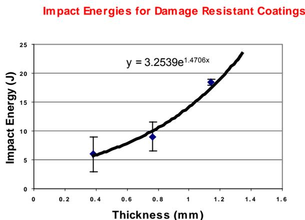
**Figure 2:** The impact values include the mean failure energy calculated using the statistical equation detailed in ASTM G14. The test results show that increasing DLFBE thickness improves impact resistance.
