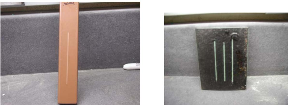
**Figure 4:** A DLFBE and a 3LPE coating was tested for gouge resistance both at thicknesses of 0.762 mm. The DLFBE retained 77% of the coating thickness while the 3LPE penetrated all the way to the steel. DLFBE has better gouge resistance than the 3LPE system. Photo courtesy of M. Mallozzi
