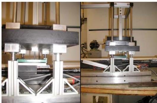
**Figure 1:** To evaluate the gouge resistance of a coating system, a coated specimen is placed on moving platform that moves at a rate of 3m/min. A normal force is applied to the coating through a stylus under a weight of 37.5 kg. The amount of gouge is measured with a depth gauge. Photos courtesy of M. Mallozzi
