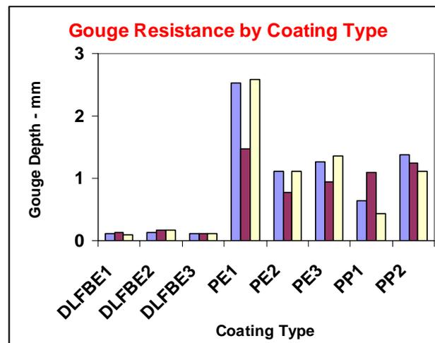
**Figure 3:** To evaluate the effect of coating type on damage resistance, a gouge test was performed with 37.5 kg of normal force. Several offerings of DLFBE showed small levels of gouge – ranging from an average of 0.16 mm to 0.35 mm, depending on formulation. PE ranged from an average of 1 mm to 2.2 mm and PP from 0.73 to 1.25.
