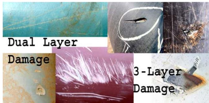
Figure 13: Properly non-motivated construction people can cause damage to either DLFBE or 3-layer pipeline coatings. Photos courtesy of J. A. Kehr, D. Norman, M. Dabiri.
