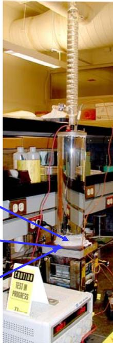
**Figure 4. When a data sheet reports a test temperature for a cathodic-disbondment test, what number is actually reported? In this test setup, one data sheet could report a 179°C test temperature, while another could report an 87°C temperature. It's important to know what is actually measured. Photo courtesy of 3M.**
