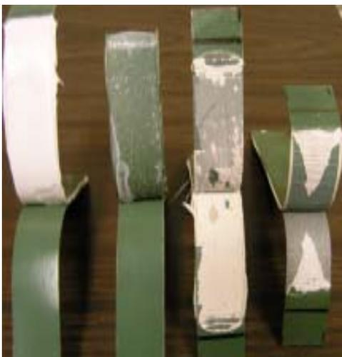
**Figure 16. Peeled Specimens from left to right: Adhesive A, Adhesive B, powder semi-ipn, Pellet semi-ipn. Cohesive failure on SEMI-IPN S, adhesive failure for adhesives A and B.**
